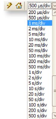
The time across the width of the display is now  $10 \times 1 \text{ ms} = 10 \text{ ms}$ , allowing 10 cycles to fit on the screen:
