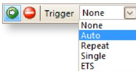
With the **Auto** trigger mode, PicoScope updates the display only when it detects a stable waveform. The display should now look like this:
