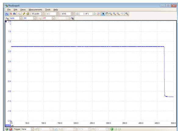
At this stage the position of the waveform is unstable because there is no trigger. We shall correct this later.
